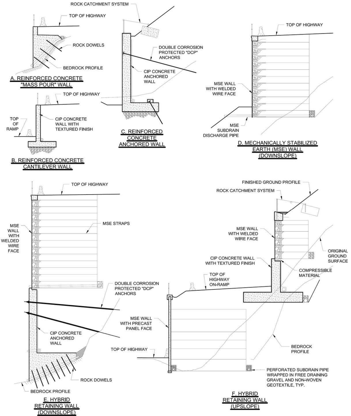
**Figure 22 – Typical Retaining Wall Combinations**
