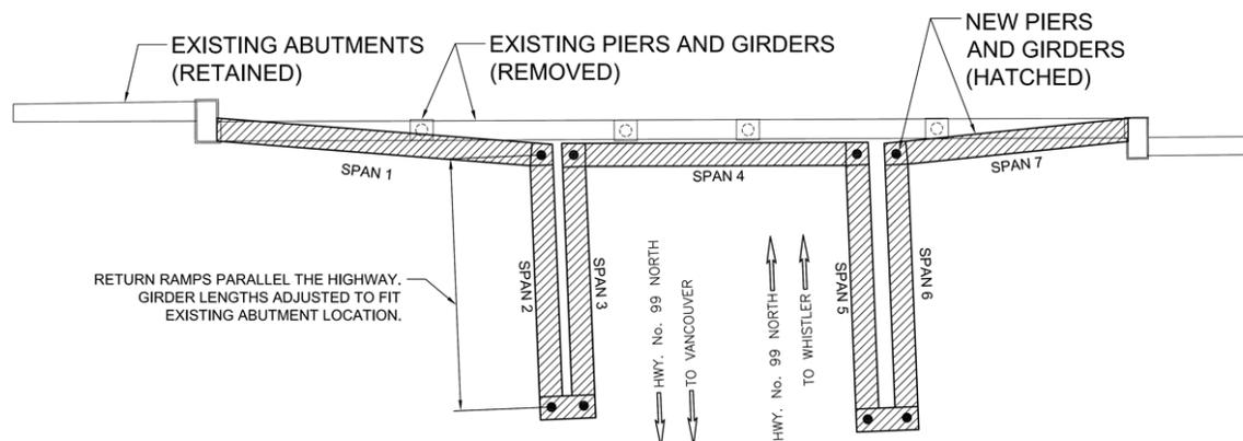
Figure 21 – Garibaldi Pedestrian Overpass - Bridge Layout
