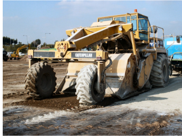
Figure 4 Pulverizing equipment used for FDR operations.
