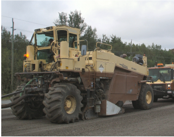
Figure 4 Pulverizing equipment used for FDR operations.
