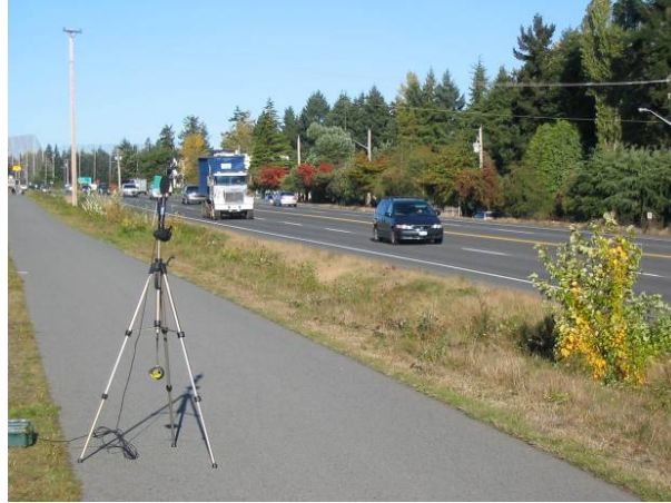
Photo 15: Sound Measurement Set-up
