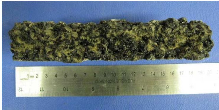
Photo 13: Side View of Core Showing Voids Filled with Debris
