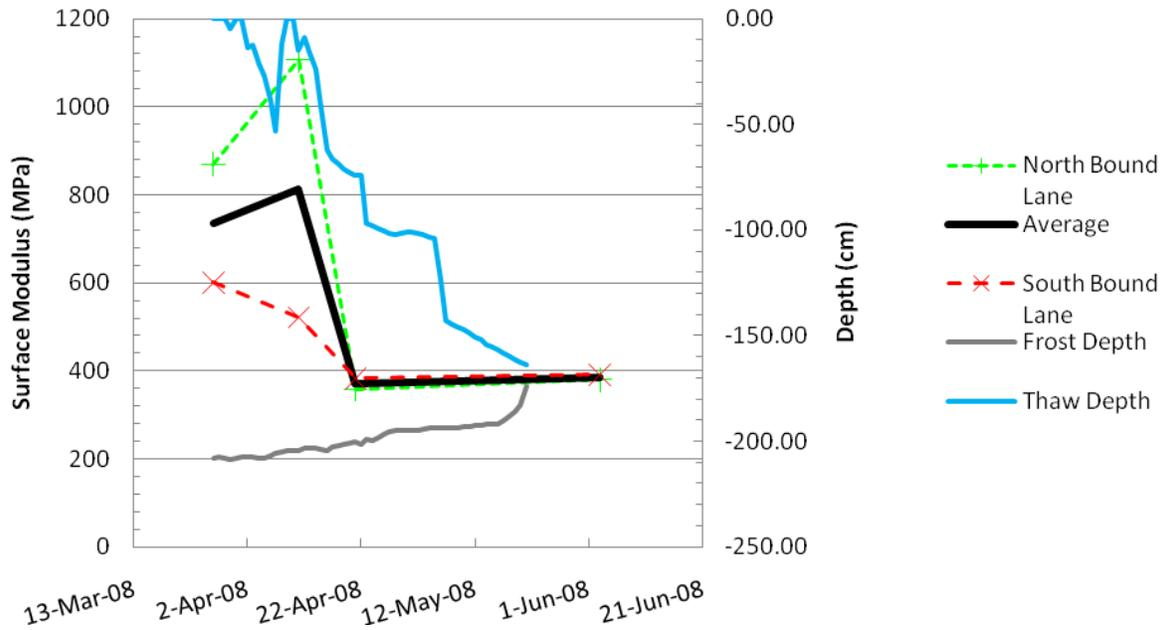
Figure 2: Surface modulus versus frost depth during spring 2008 at the Highway 527 site (Al-Mahdawe et. al. 2009)
