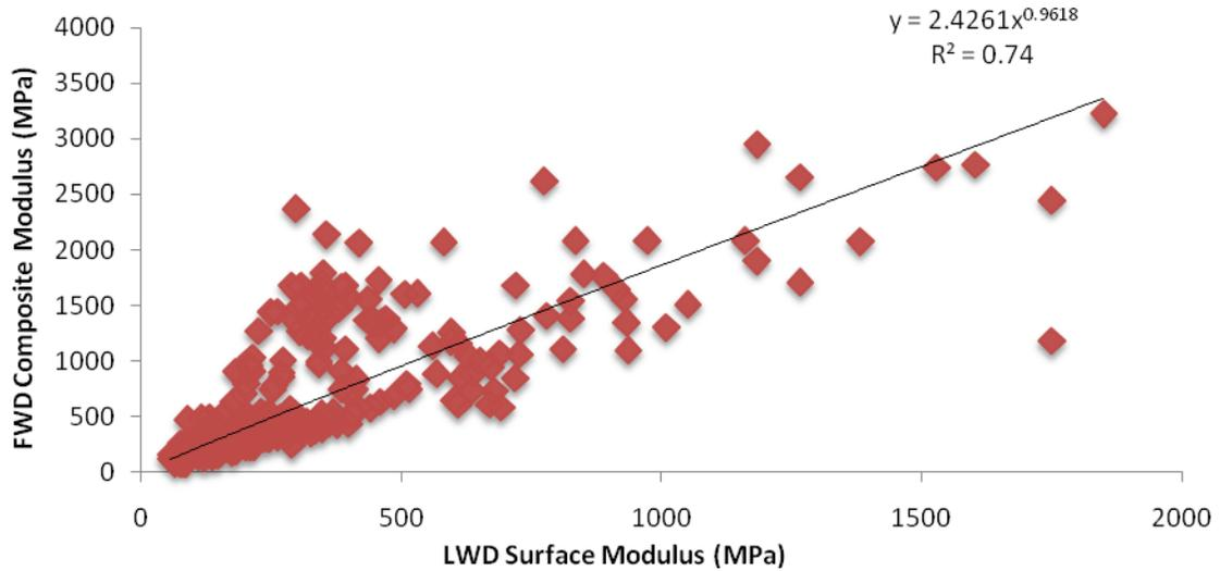
**Figure 5: LWD/FWD surface modulus comparison of all Northeastern Ontario data excluding values >3500 (Al-Mahdawe et. al. 2009)**
