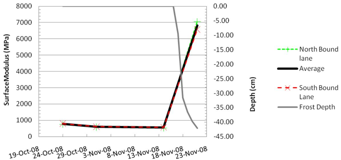
Figure 3: Surface modulus versus frost depth during fall 2008 at the Highway 527 site (Al-Mahdawe et. al. 2009)
