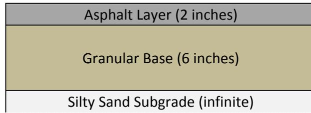
**Figure 6: Typical Low Volume Road Pavement Structure used in ME-PDG analysis (Al-Mahdawe et. al. 2009)**
