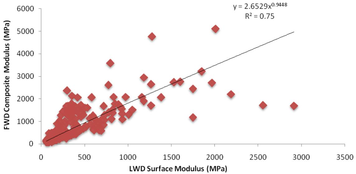
**Figure 4: LWD/FWD surface modulus comparison of all northeastern Ontario data (Al-Mahdawe et. al. 2009)**
