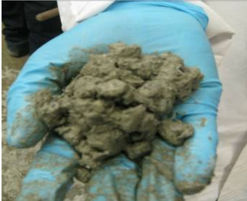
Figure 2: Testing the Pervious Concrete for Consistency
