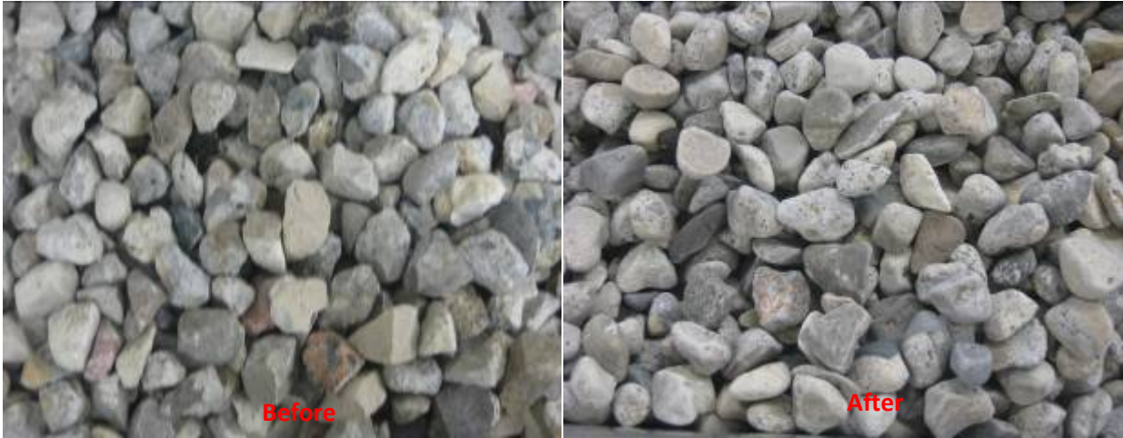
Figure 11: RCA before and after the Micro-Deval Abrasion Test
