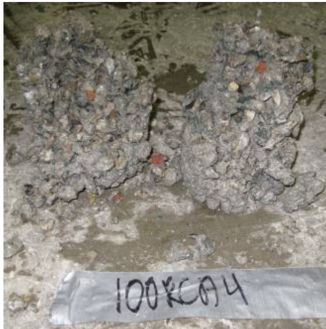
Figure 5: Failure Plane of the 100RCA Samples
