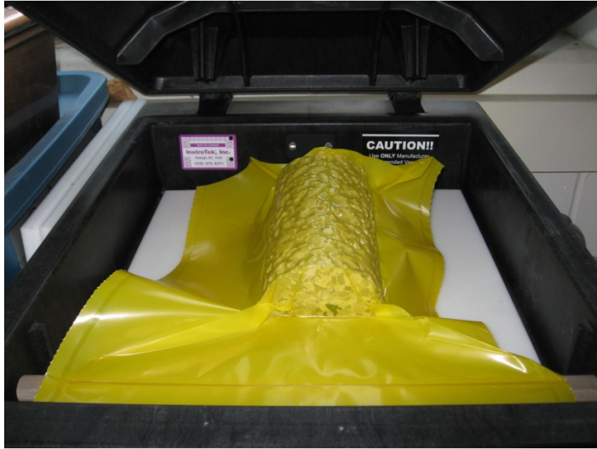
Figure 6: Vacuum Sealed Specimen to Test for Void Content
