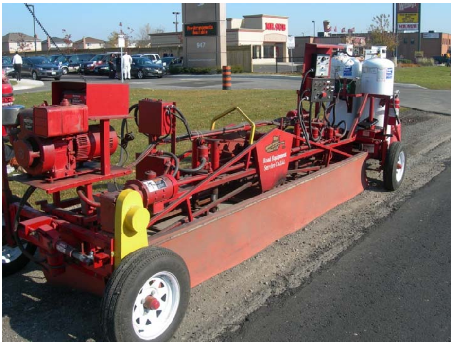
Photograph 3 Infrared joint heater used on paving projects in Hamilton in 2008.
