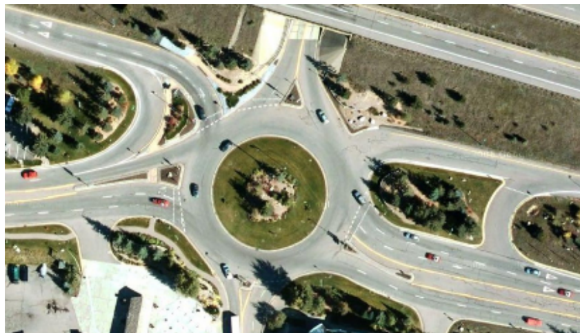
Figure 3.6 Free-Flow and Yield-Controlled By-Pass Lanes
