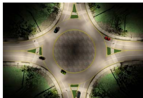
Figure 11 - Approach Mounted Lighting 8-250W HPS (Courtesy: DMD Associates, Canada)
