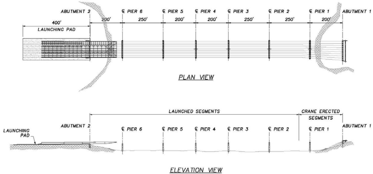
Figure 8. Schematic view of erection concept
