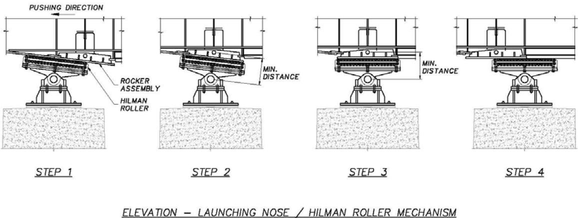
Figure 10. Rocker assembly working mechanism
