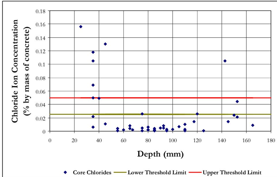
Figure 7: Chloride ion concentrations vs. depth.
