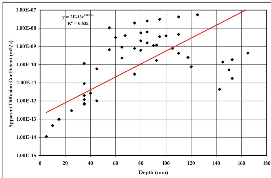
Figure 8: Correlation between diffusion coefficient and depth from surface (diffusion coefficient in log scale).
