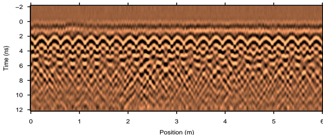
Figure 2: Typical section of bridge deck data without distresses.
