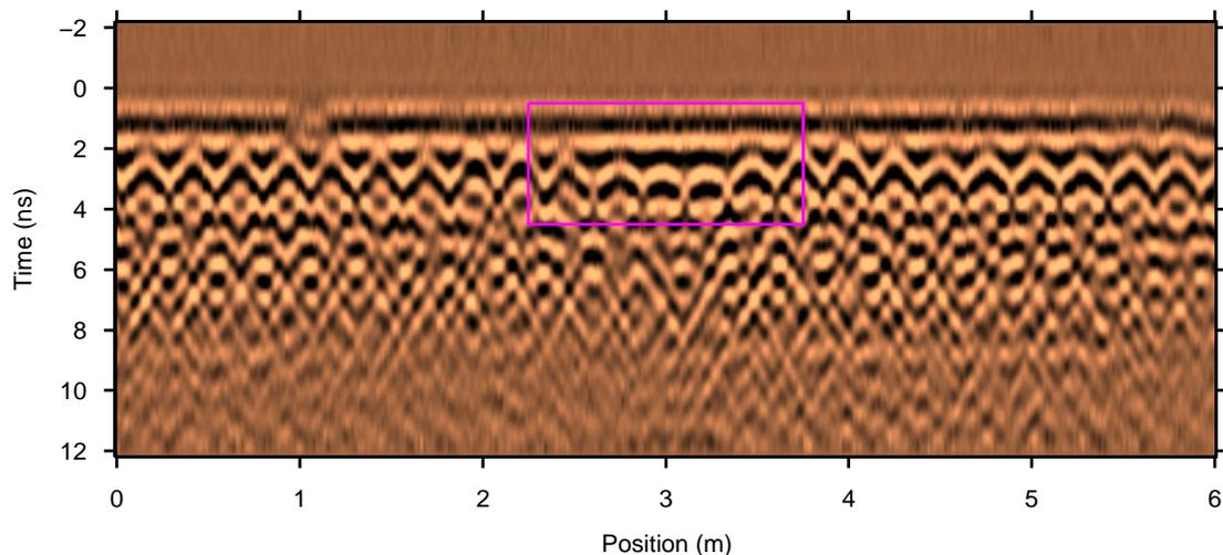
Figure 3: Bridge deck radar data showing an area with rebar distress signatures.
