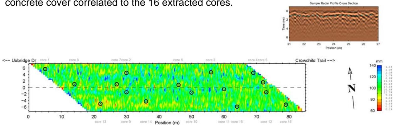
Figure 4: Steel-fibre PCC cover plan map.
