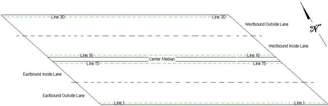
Figure 1: Survey line layout (not to scale).
