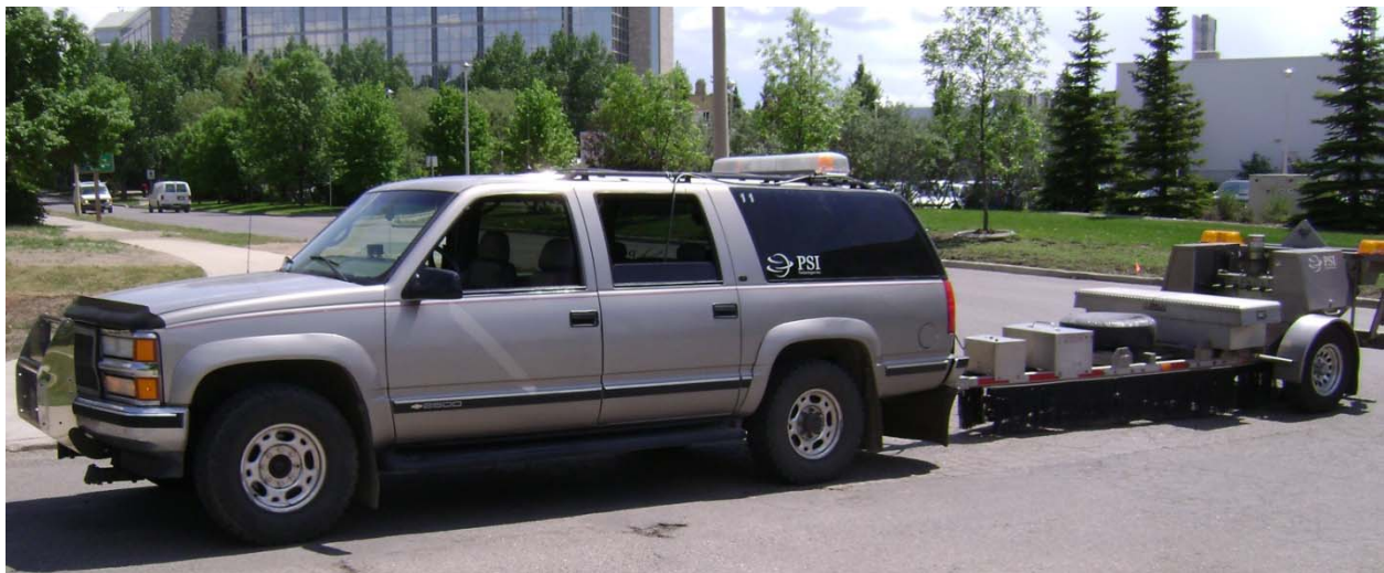
Figure 9 PSI Technologies Heavy Weight Deflectometer on North Road
