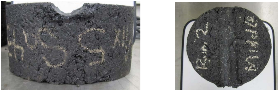
Figure 2 Specimens after APA testing
