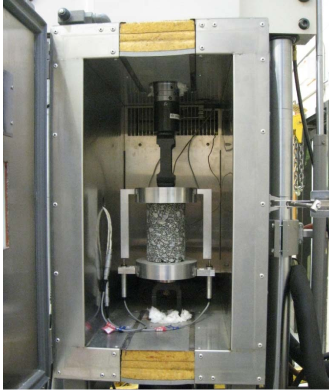
Figure 3 Dynamic modulus testing in an environmental chamber
