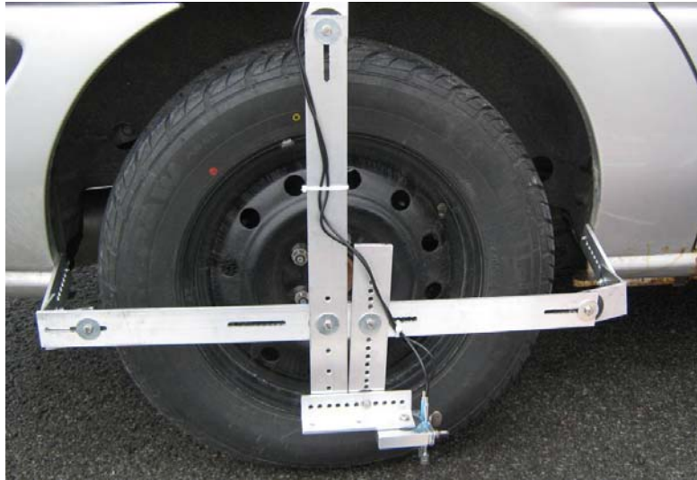
Figure 9 - Sound intensity probe mounted on test vehicle at leading edge of tire contact patch
