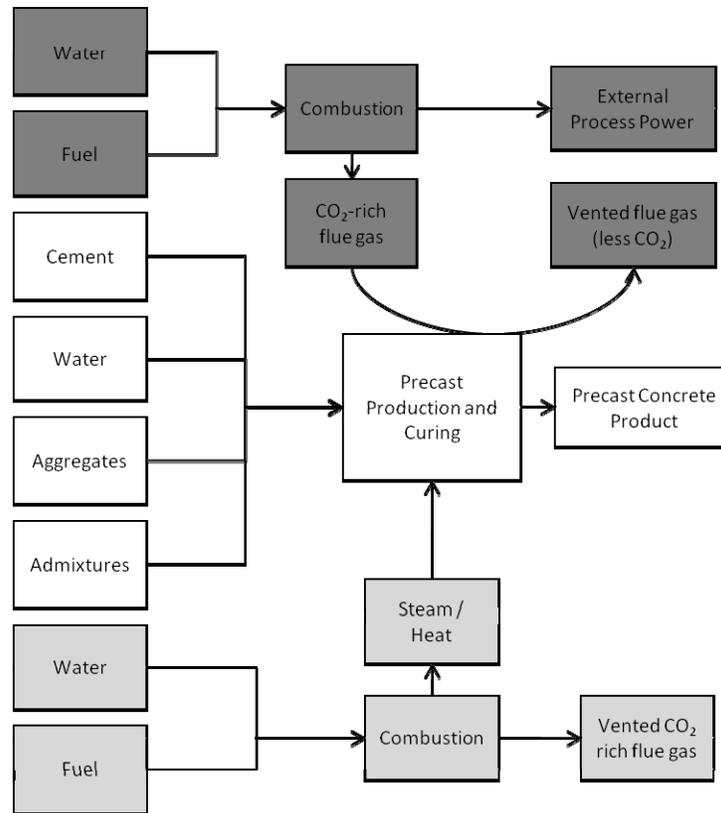
Figure 1. Block diagrams of the CO<sub>2</sub> Accelerated Concrete Curing process (top, hatched) and conventional steam curing process (bottom, dark). Both processes share the common concrete production process (middle, no fill).
