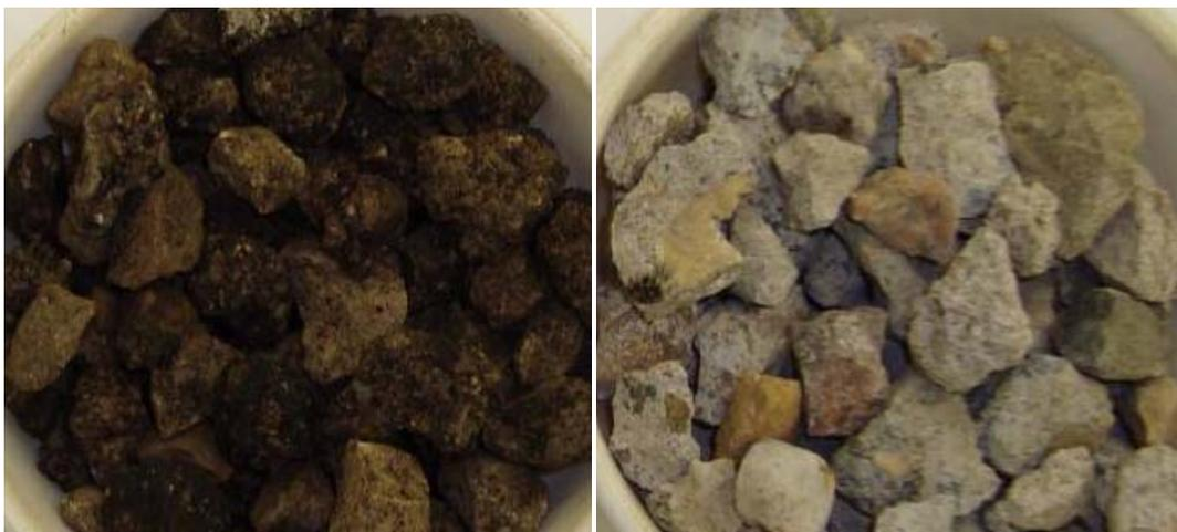
**Figure 7 Second generation impact crushed HMAC and PCC material (OGBC)**
