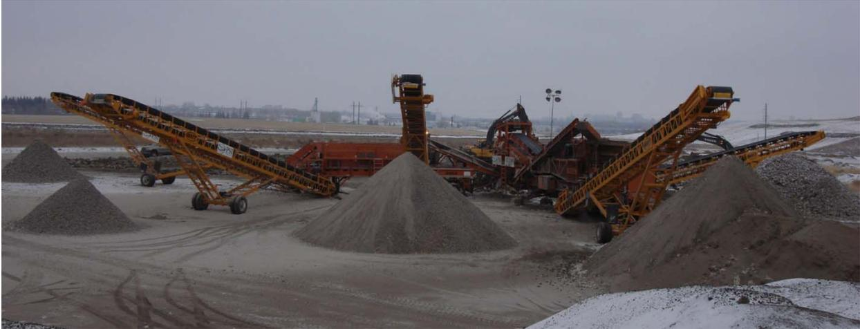
**a) Crushed reclaimed HMAC material**
