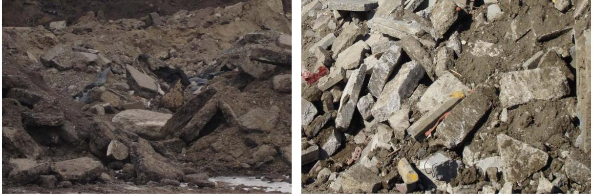
**Figure 1** Stockpiled HMAC rubble (left) and stockpiled PCC rubble (right)
