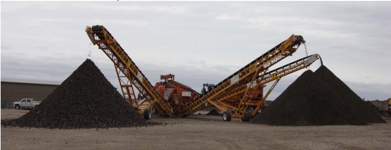
**b) Crushed reclaimed PCC material**
