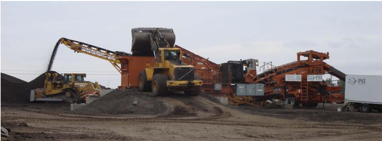
**Figure 4** Reconfigured impact crusher (2009)
