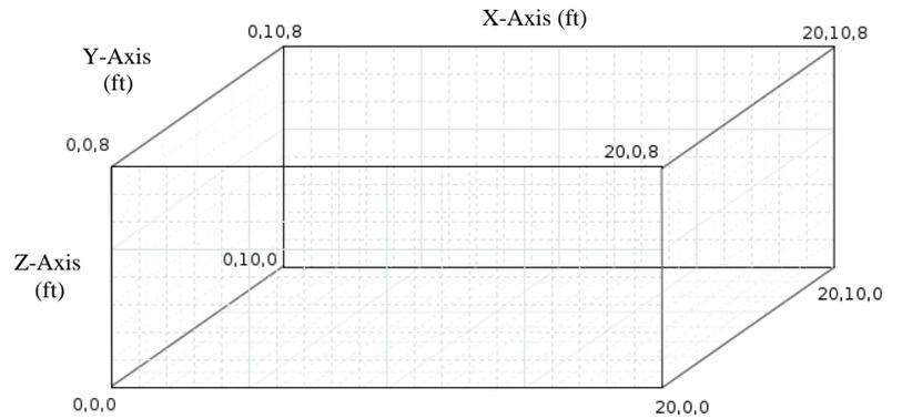
**Figure 1. Soil Box provided by FDOT**
