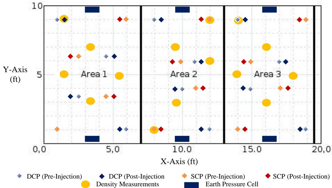
**Figure 4. Location of DCP/SCP Testing**
