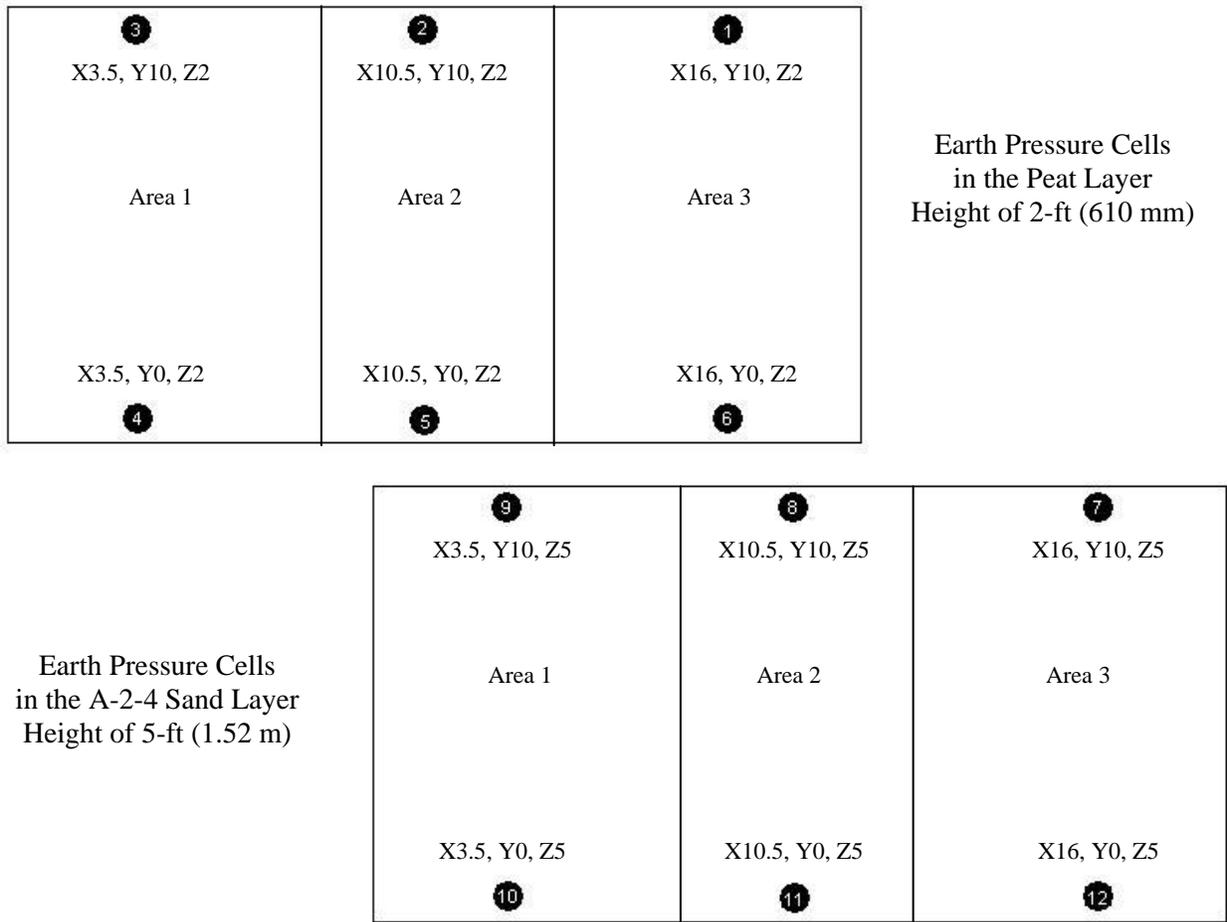
**Figure 6. Coordinate Locations of Earth Pressure Cells**
