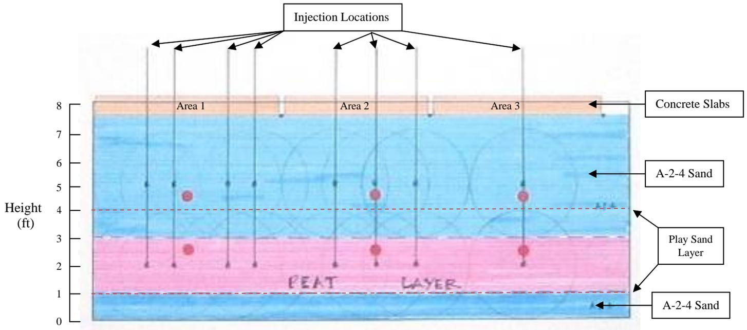
**Figure 3. Constructed Pavement Structure (After Consolidation of the Peat Layer)**
