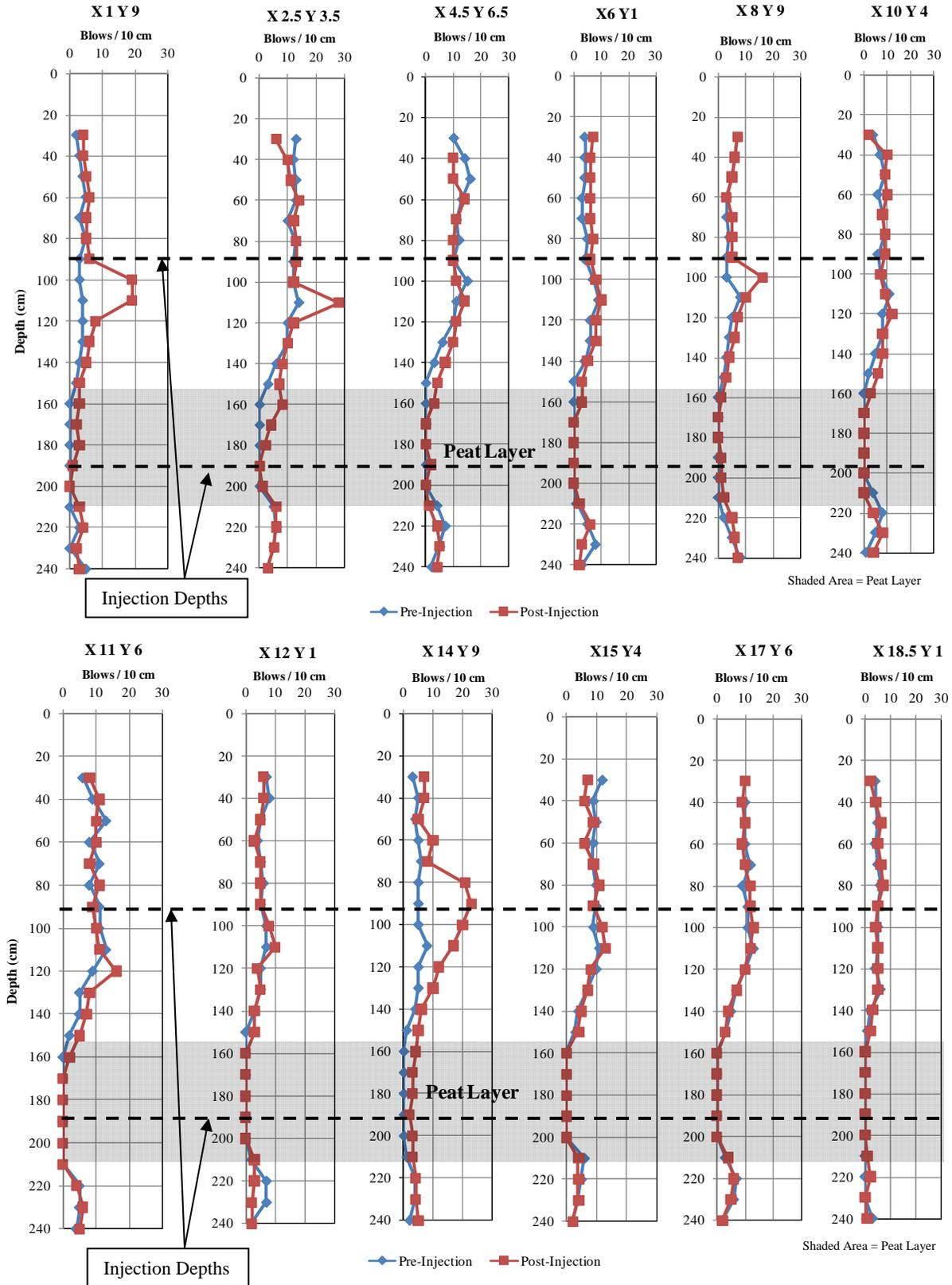
Figure 9. Comparison of DCP Test Results (Pre-Injection and Post-Injection)
