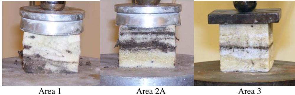
**Figure 10. Photographs of Representative Samples for Compressive Testing**
