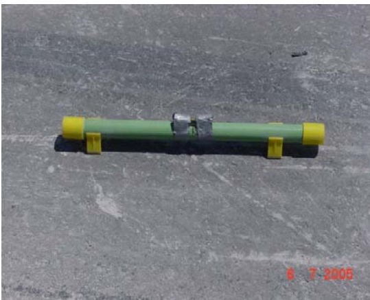
Figure 9 Highway 417 Westbound Dowel-Bar retrofit
